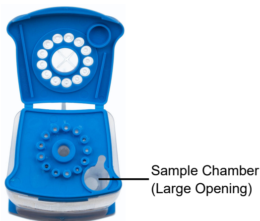
Figure 15. Xpert Xpress CoV-2/Flu/RSV plus Cartridge (Top View)
