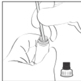
SAMPLE LOOP INSERTED INTO DPP SampleTainer BOTTLE
